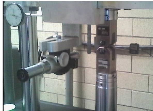
Fig. 2. Specimen and extensometer mounting.
